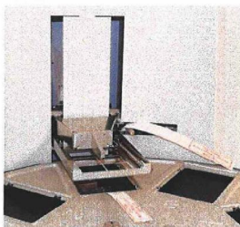
Figure 31 Both transport locks refitted
